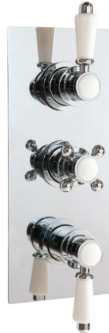
Thermostatic Shower Valve: 1 Water Flow With Diverter For Two Separate Outlets, 2 Temperature, 3 Water Flow Single Outlet (1 And 3 Can Be Used Separately Or Simultaneously)
